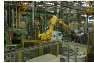
Gravity die casting cell
